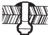
SEALED End of rivet is sealed for weatherproofing
