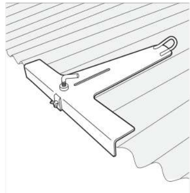
Sit the anchor on top of corrugation roofing iron as shown
